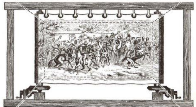
The machinery for a moving panorama ( Scientific American , 1848)
