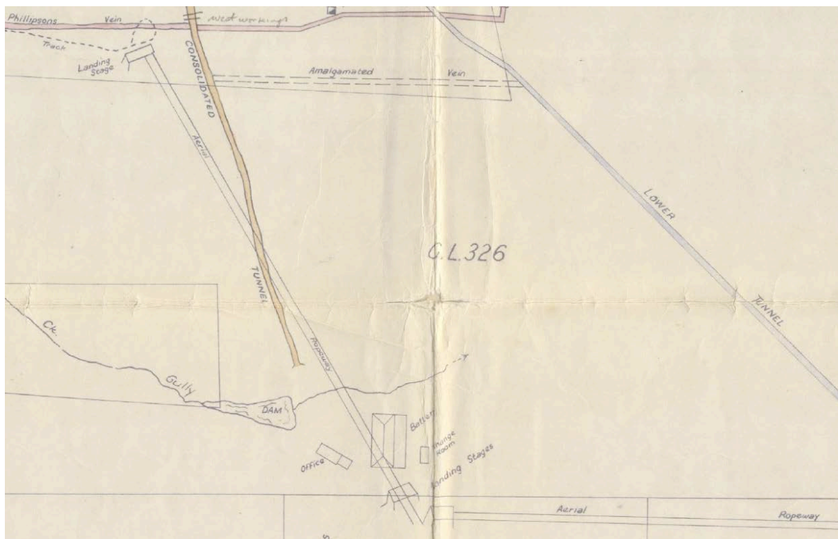
Figure 11: Detail from a 1950 Plan of Workings at Hill End N.S. Wales prepared by J.T. Paul Jones. This shows the line of the aerial ropeway from Hawkins Hill to the Consolidated stamper in Nuggetty Gully. A second aerial ropeway ran along the side of Prince Alfred Hill. (Marshall's Gold Reward Hawkins Hill [Online])
